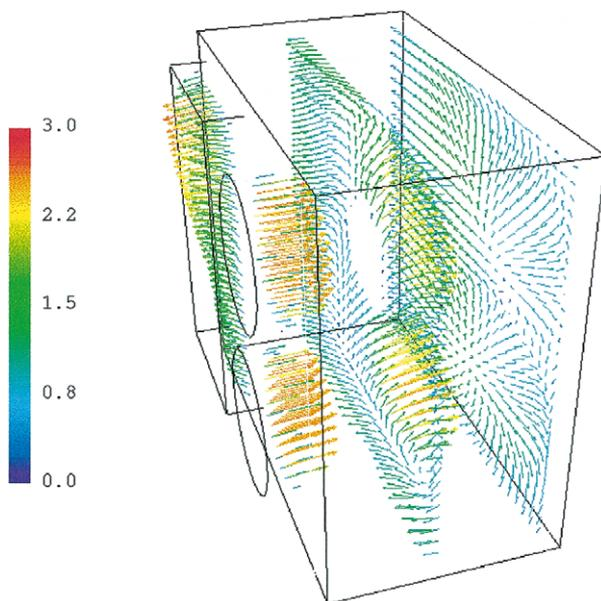
Fig. 2. An example of the flow field in the chiller shown in Fig. 1 predicted by CFD code (Hu and Sun, 2000b).
