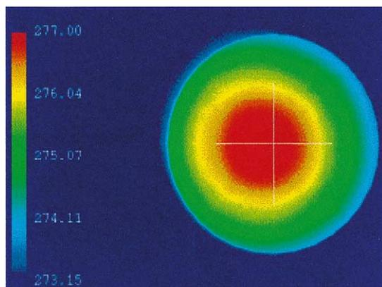
Fig. 3. An example of temperature distribution of the ham during chilling in the air blast chiller shown in Fig. 1 (Hu and Sun, 2001b).
