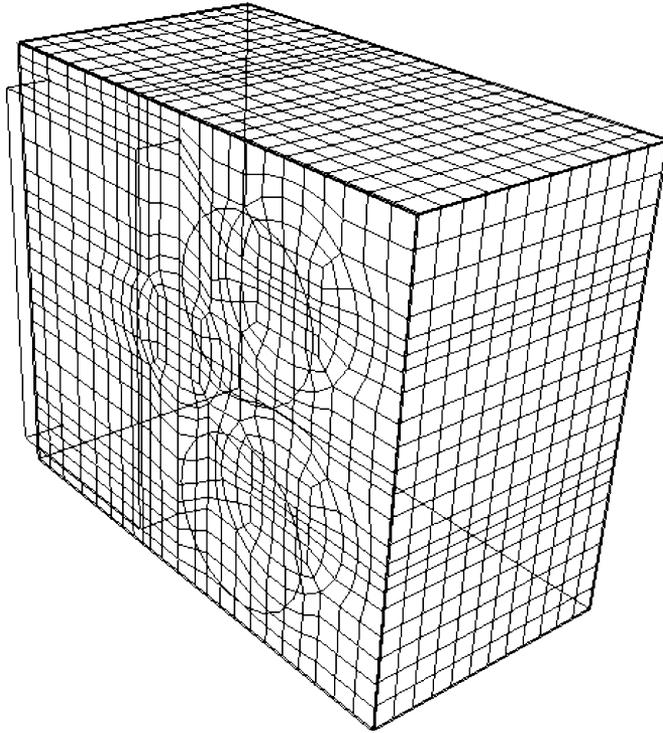
Fig. 1. Meshing structure of a commercial air blast chiller with a ham inside (Hu and Sun, 2001b).
